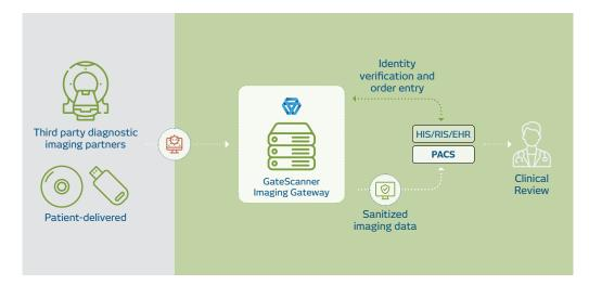
**GateScanner® Imaging Gateway** provides a simple path to securely receive DICOM files from external sources. GateScanner's advanced, deep deconstruction capability analyzes every DICOM file, removing any non-DICOM content and attached executables while strictly maintaining the clinical integrity of the core imaging data.
