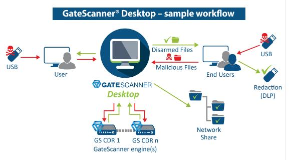
Users insert portable (USB) devices at the endpoint, activating a desktop application, which sends the files to a networked GateScanner service. The disarmed files are then saved to a network location. Files can be securely exported using Redaction (DLP) policies.
